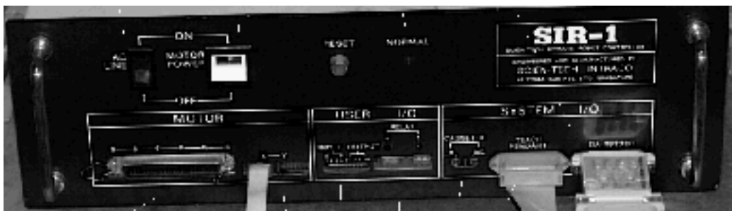
Figure 2. The Serial Port to Stepper Motor Controller
